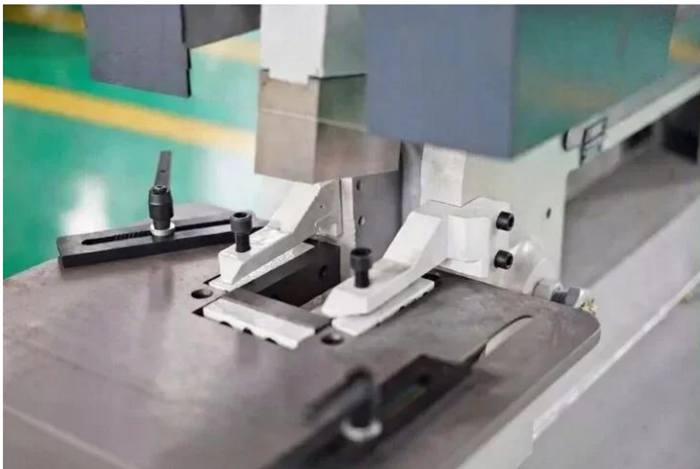
Hydraulic sheet shears – material cutting up to 50 mm
